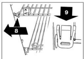
Slide the plastic plugs into the holes of the wall. Snap the shelf locks onto the wire shelf.
